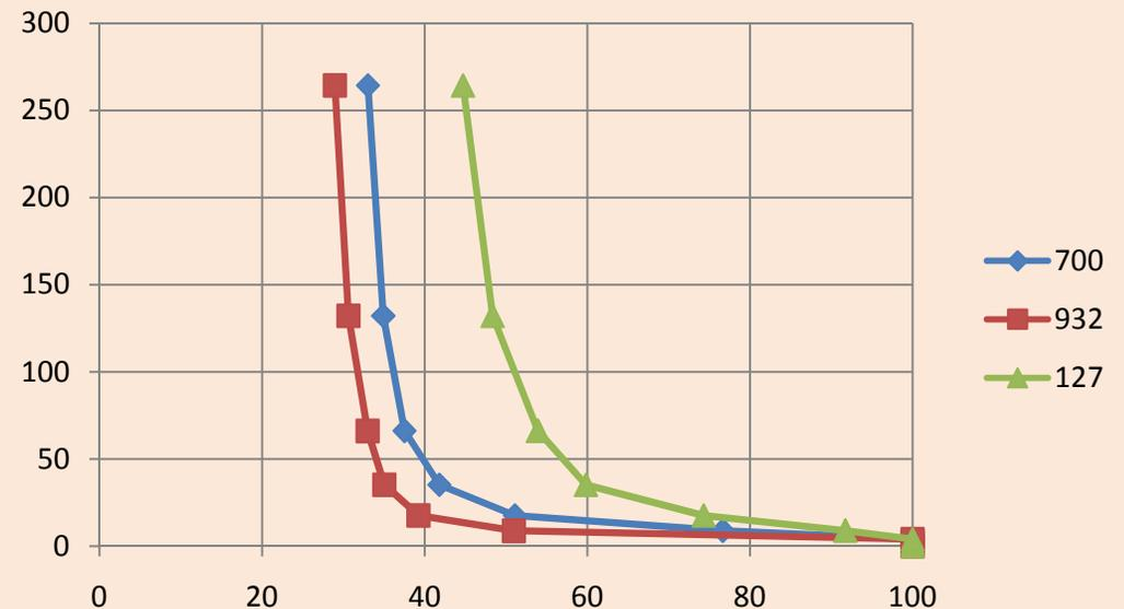
Capillary pressure curves have a characteristic shape as shown above. They also have a characteristic ordering, in which higher permeability samples have a lower  $S_{wirr}$  than lower permeability samples. The entry pressure (and therefore entry height) is also higher for low-perm rocks.
