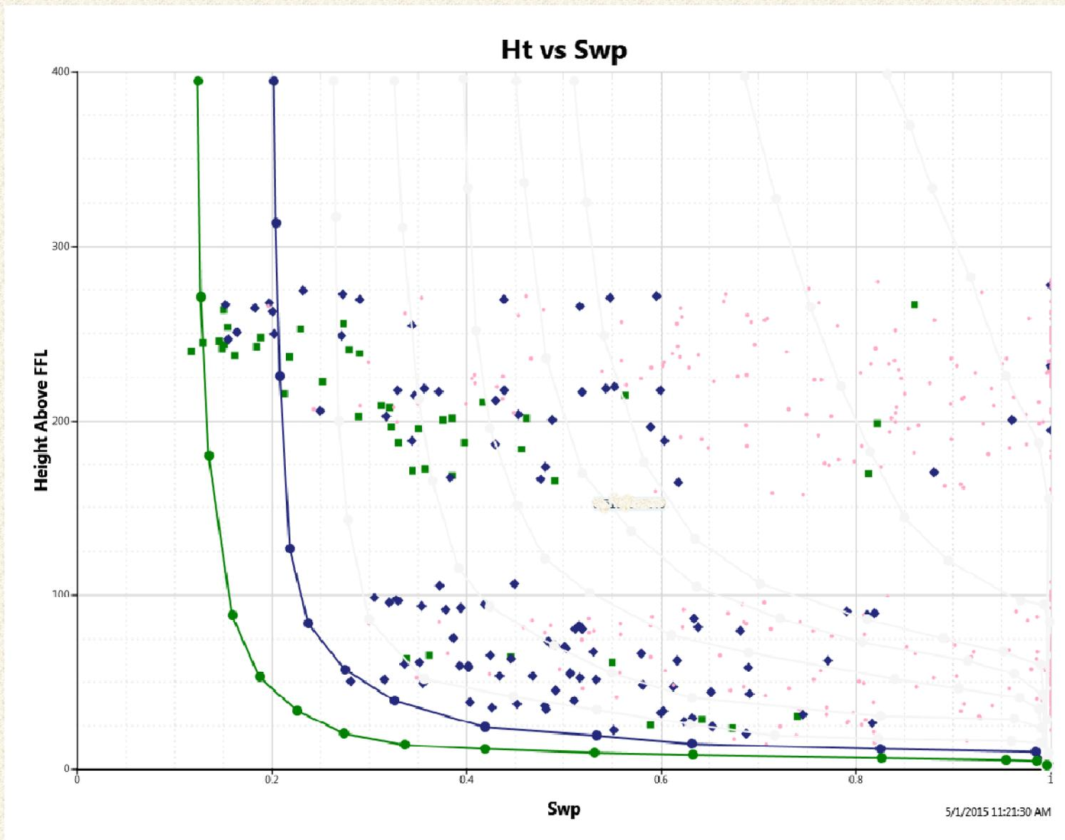
Data between 500-1500 md (blue) area added, with fitted curve = 1500md. A few low-Sw points are ignored. Sample failure and other analytical problems can be common in unconsolidated sands.
