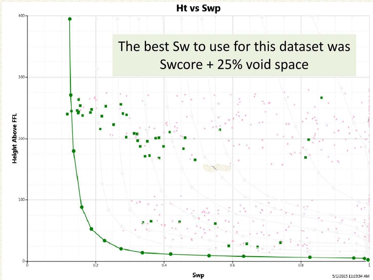
When the correct Sw and the most representative permeability ranges have been chosen from the data, highlight them on the Sw vs Ht plot. Green dots are data with  $k > 1500$ , and a curve is fitted to the high end of the distribution. The curve represents 5000 md permeability and is intended to bound the model at the high end.
