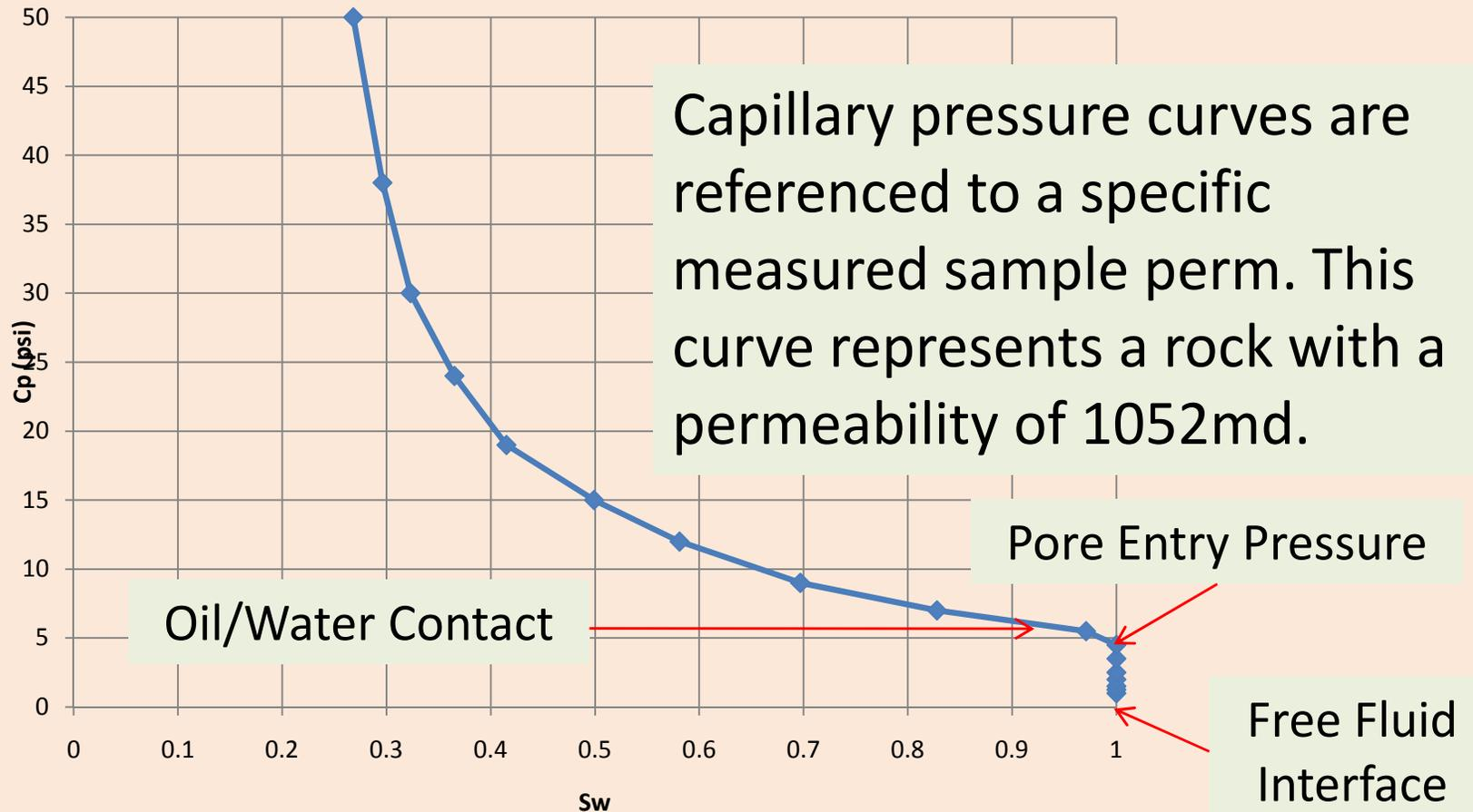
After reaching pore entry pressure, oil enters the system and begins to displace water ( $S_w$  decreases). The process is initially rapid, then as pressure continues to increase less and less water is displaced.
