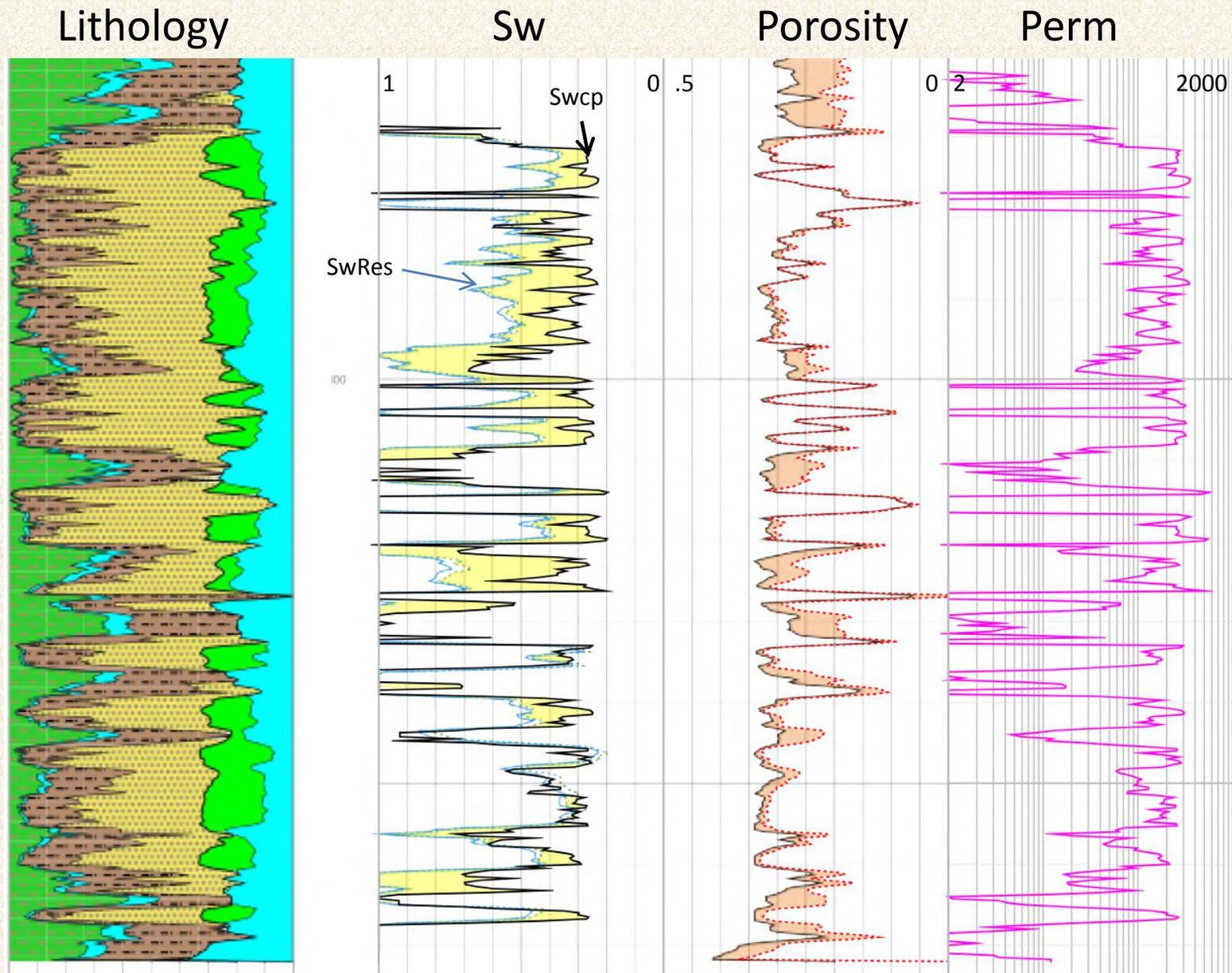
Comparison of Sw from resistivity logs (blue) with Swirr from pseudo-capillary pressure curve set (previous slide). Log-derived permeability curve (pink) was the reference used to enter the Cp model.
