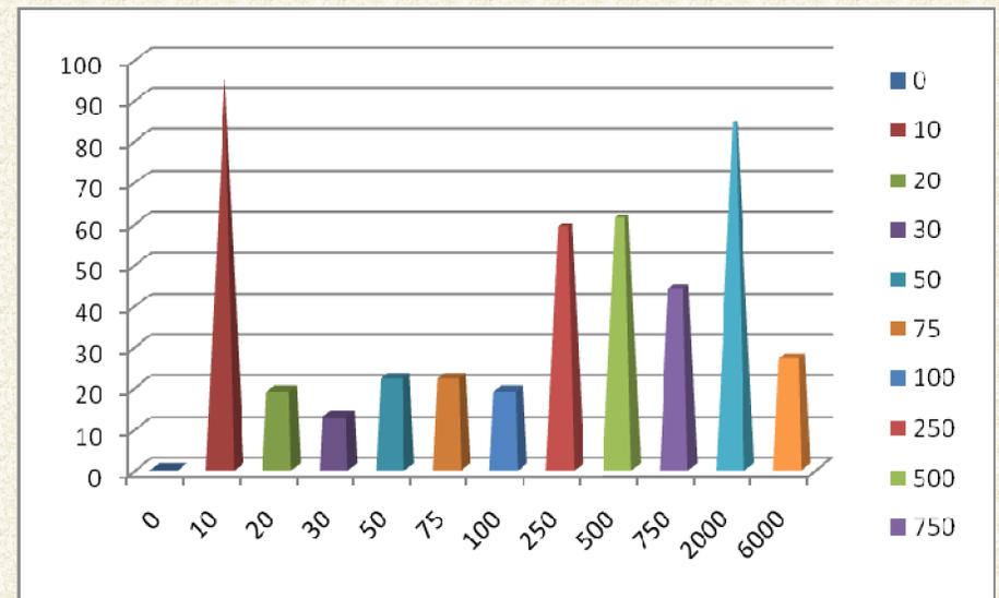
Divide the core data into various permeability bins to see what the distribution is. This dataset is dominated by low and high values, with a moderate distribution in the 250-750 range. These ranges will determine the groupings on which the psuedo-Cp curves are based.
