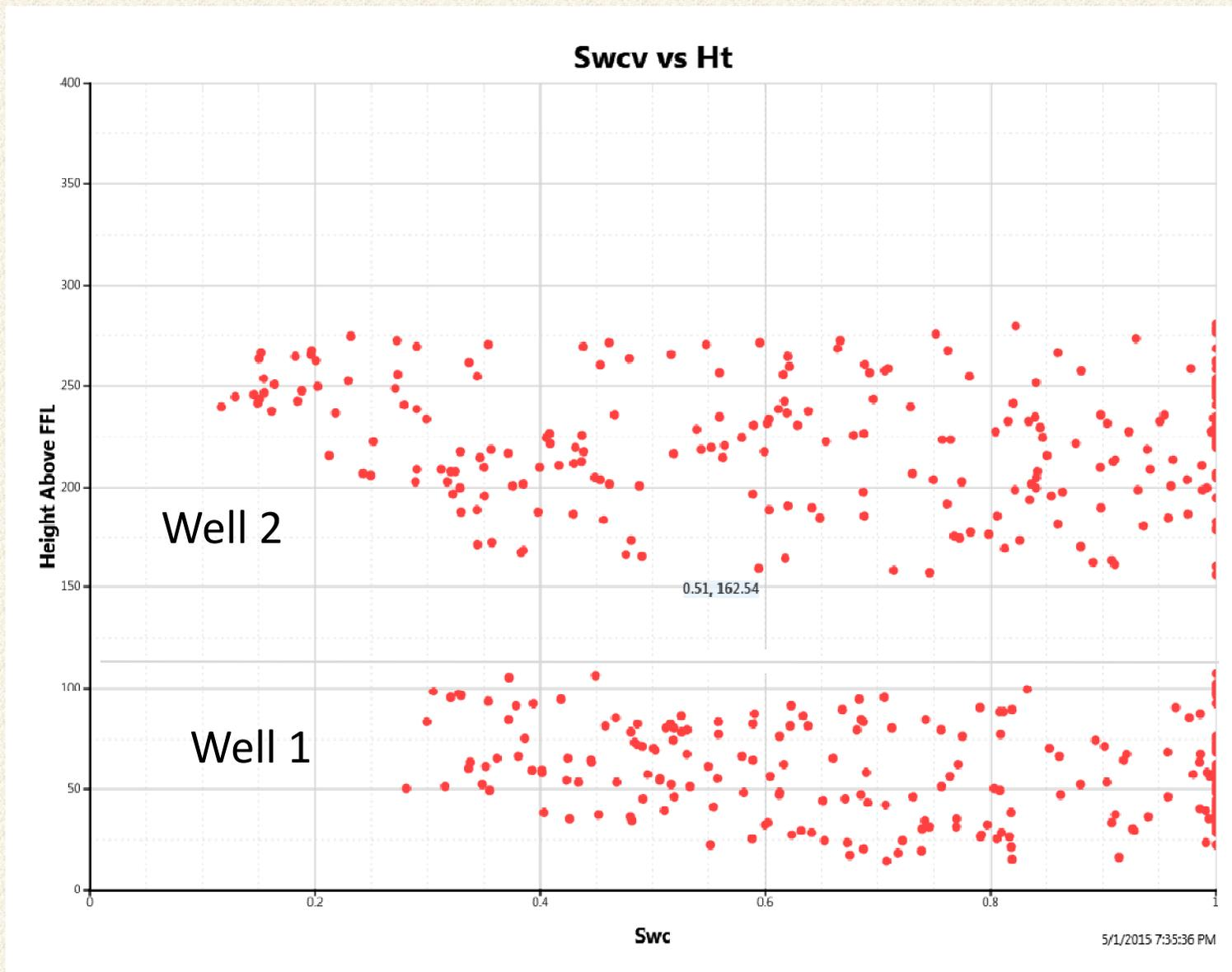
This is a core dataset with two wells at different heights above the oil/water contact. The data suggest that Well 1 is not as high on the capillary pressure curve as Well 2.
