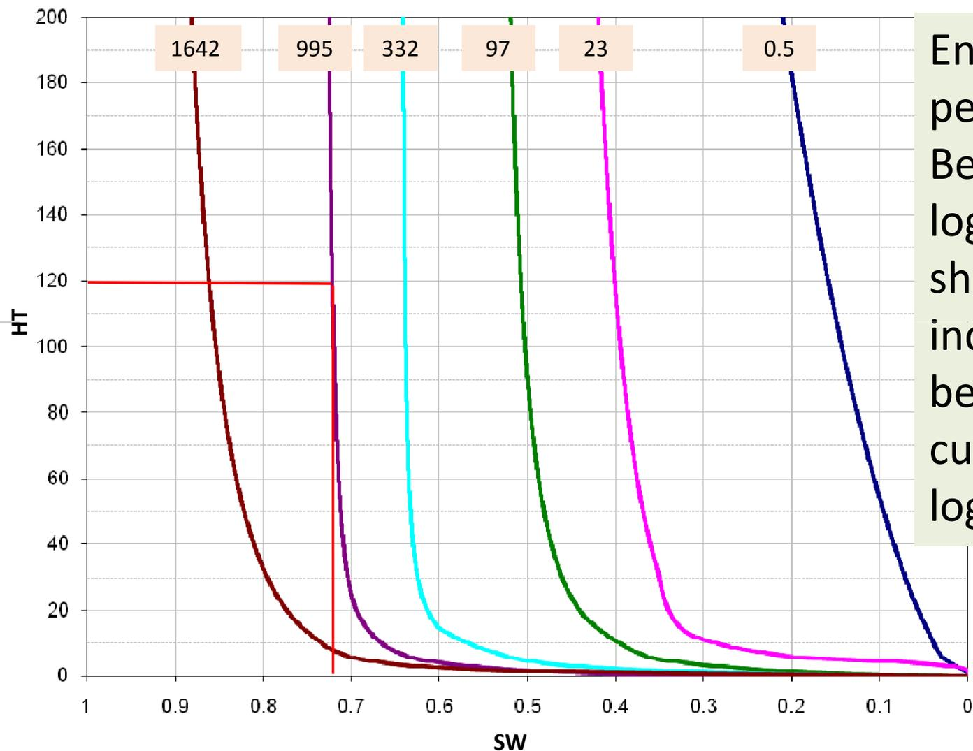
Enter with Ht 120' at perm 995, Sw = 72%. Because perm has a logarithmic relationship to other indicators, interpolation between permeability curves is not linear but logarithmic.
