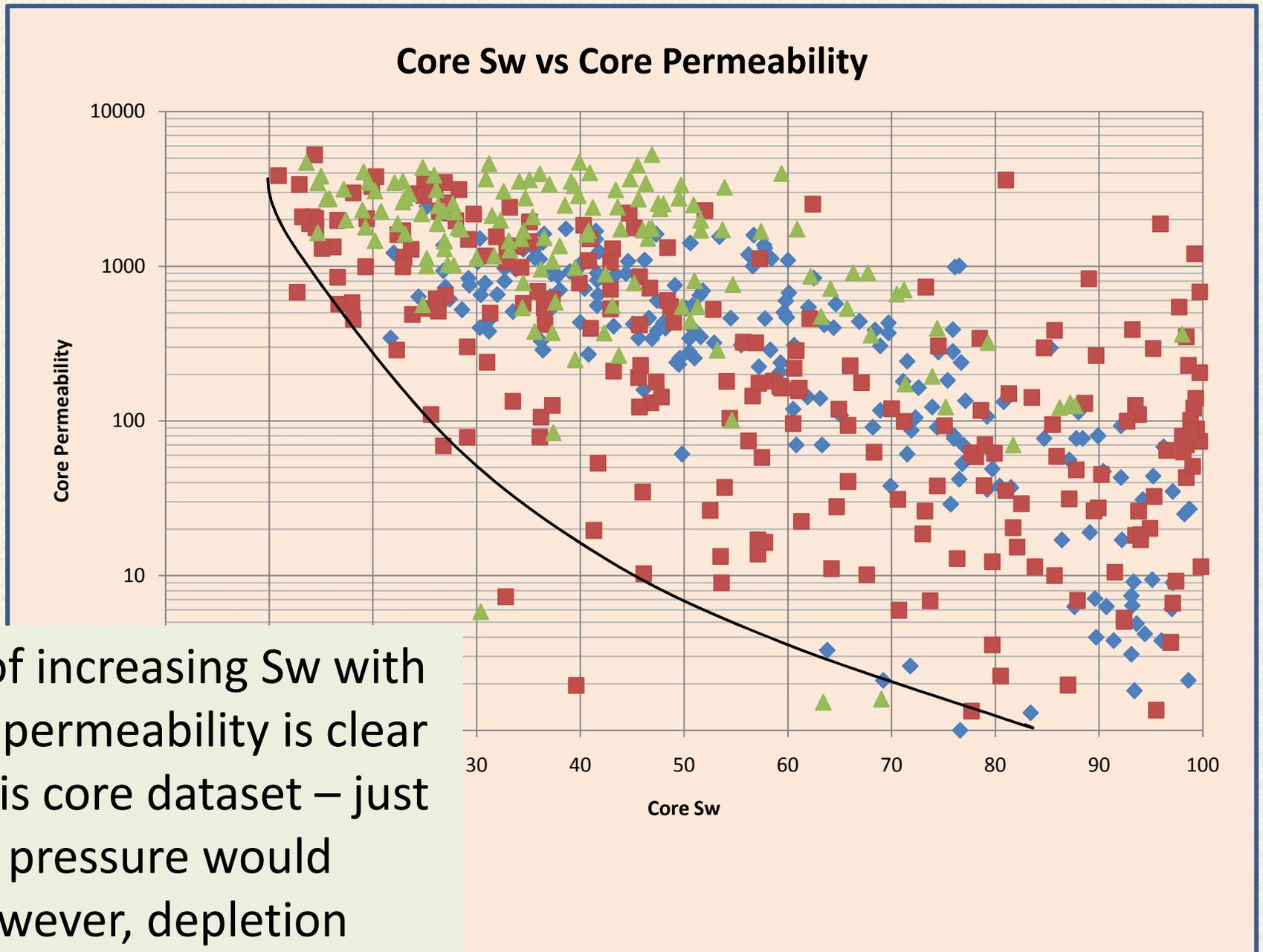
The trend of increasing Sw with decreasing permeability is clear to see in this core dataset – just as capillary pressure would predict. However, depletion trends are also obvious in the data spread from left to right.
