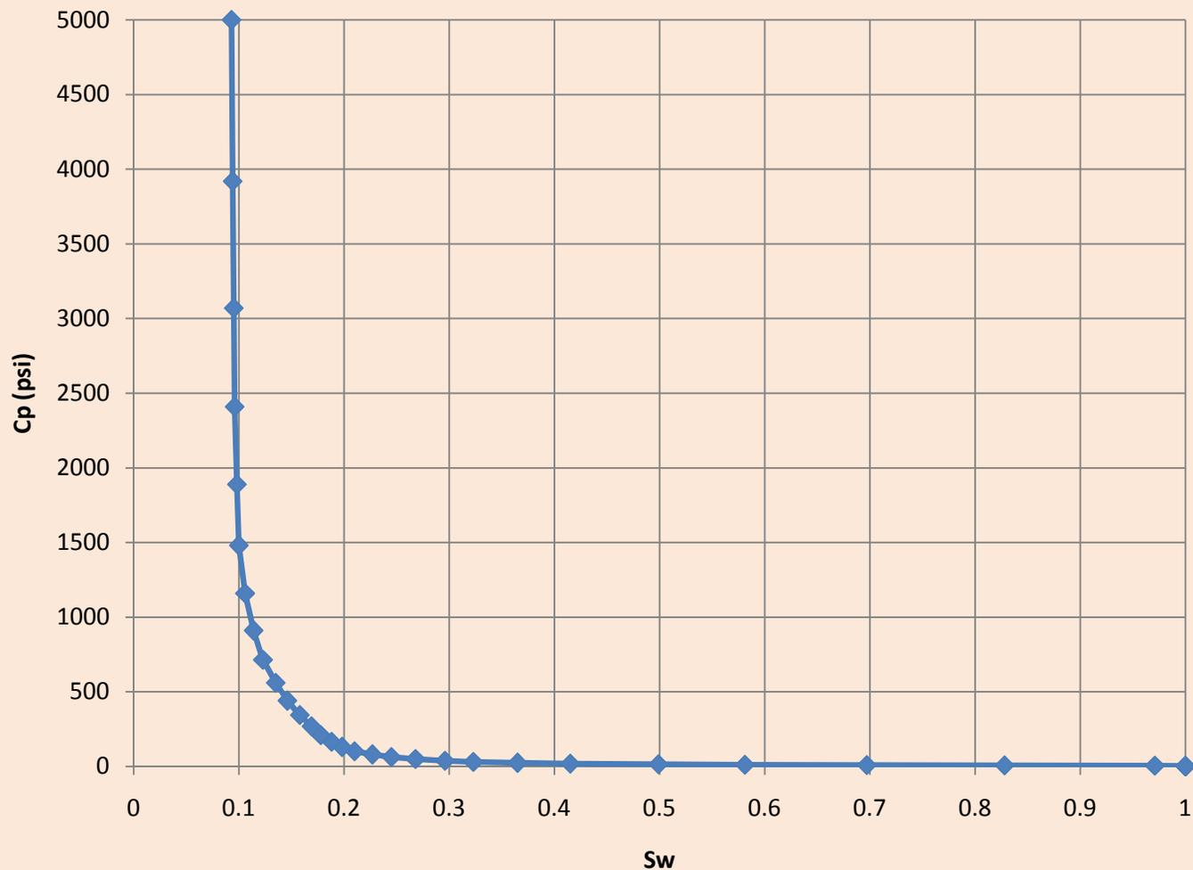
Above a certain pressure, very little additional water is displaced and the curve become asymptotic. The minimum Sw reached is equivalent to the irreducible Sw at that permeability.
